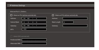
④ Go to Start → Settings → Camera → Add Camera. The NVR will automatically refresh the cameras searched. The IPC which supports the Onvif protocol may be added manually. If the IPC searched is not in the same local network as the NVR, you should select the device and click ■ to modify the IP address.
