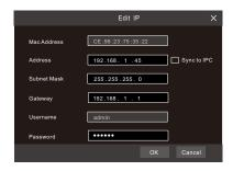
⑤ Checkmark the device you want to add and then click "Add" button. The NVR will automatically refresh the cameras and return to "Edit Camera" interface. "Online" status means connecting the device successfully and you will see the live image. You may select the added device and click ■ button to modify channel, IP address, ect.
