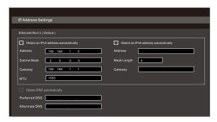
④ Go to Start → Settings → Camera → Add Camera. The NVR will automatically refresh the cameras searched. The IPC which supports the Onvif protocol may be added manually. If the IPC searched is not in the same local network as the NVR, you should select the device and click ■ to modify the IP address.
