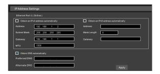
③ Go to Start → Settings → Camera → Add Camera. The NVR will automatically refresh the cameras searched. The IPC which supports the Onvif protocol may be added manually. If the IPC searched is not in the same local network as the NVR, you should select the device and click to modify the IP address.
