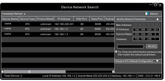
③ Modify the IP address. The default IP address of this camera is 192.168.226.201. Click the information of the camera listed in the above table to show the network information on the right hand.
