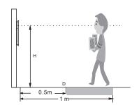
• The recommended installation height (H) is 1.45m. It can be adjusted according to the actual scene. The ideal face recognition distance(D) ranges from 0.5m to 1m.
