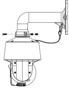
3. Drill the screw holes on the wall according to the drill template. Then insert the plastic plugs into the holes. 4. Insert two screws to the holes as indicated by the arrows (left) and leave 12mm clearance.
