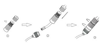
(1) Loosen the nut from the main element.
